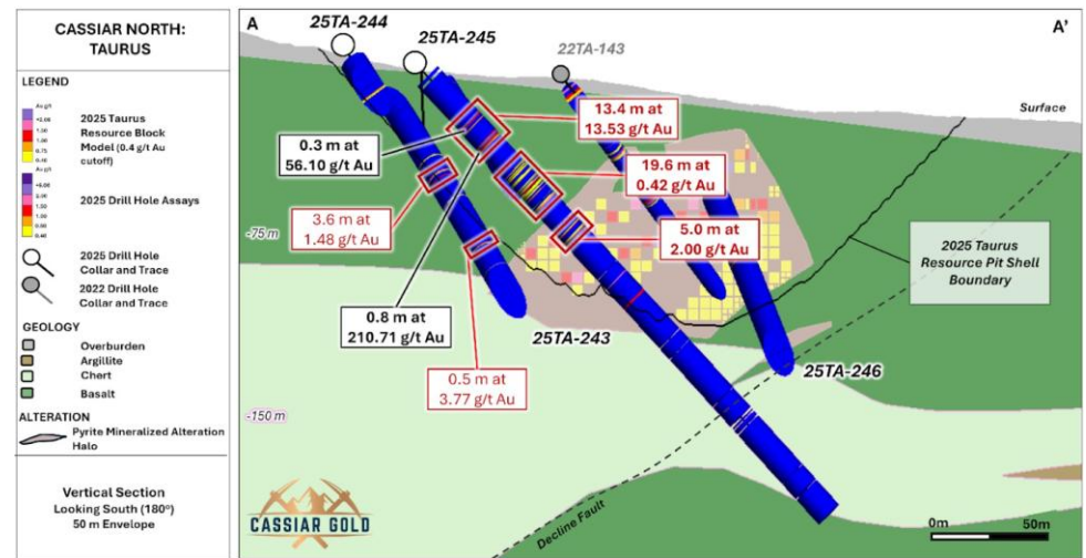
Figure 3: Vertical section of drill hole 25TA-245 at Taurus East, looking to the south
