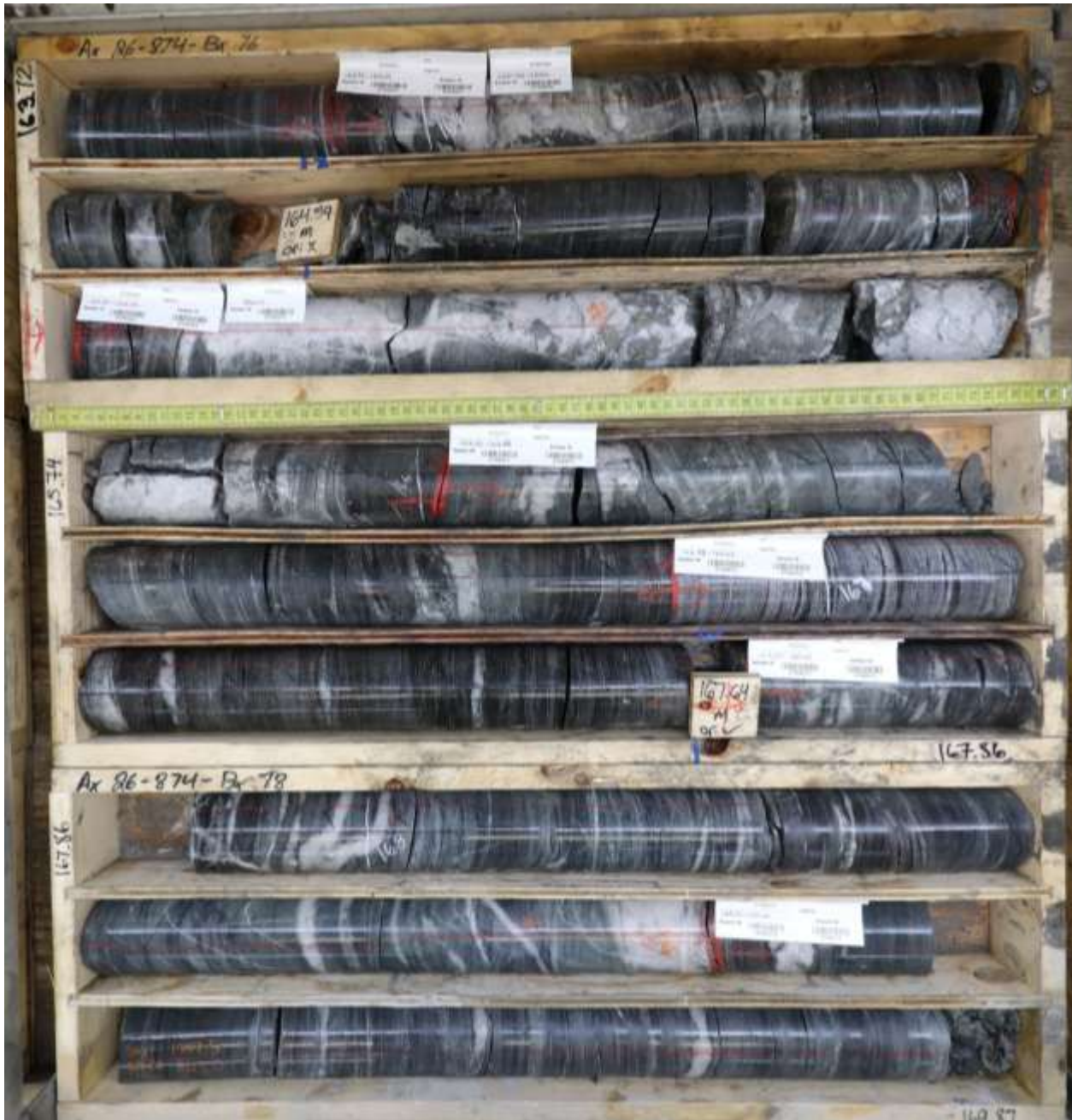
Figure 5: Mineralized extensional quartz veins in metasedimentary rocks in Powerline North from diamond drillhole AX-26-874. High density of extensional quartz veins with bismuth-sulphosalts, arsenopyrite, and pyrite found throughout the mineralized interval from 160.0-174.2m, which graded 13.03 g/t Au over 14.2m and hosts several instances of visible gold mineralization (Figure 6). Locally, very high-grade gold intersection of 142.70 g/t Au over 1.0m is associated with locally brecciated quartz extensional vein with coarse-grained to semi-massive arsenopyrite.
